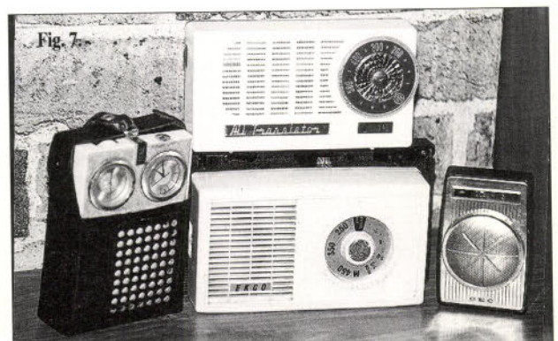
Fig. 7: Collectable transistor receivers. (Left) the Russian-made 'Signal 601' with wind-up watch type alarm. The Ekco (bottom) tunes through the medium wave band and 'clicks' into a preset 'Light' programme on the long waves (now BBC Radio 4).
